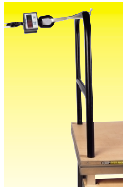
MultiRel railing in lateral-load test up to 100 kg/m.
