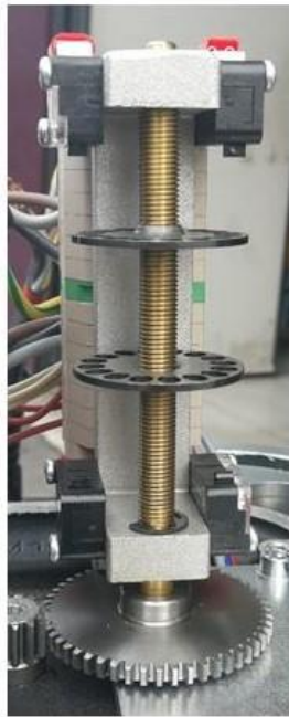
figure 3.14 – “Settings for 2 and 2+2 position limit switches”
