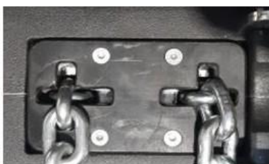
figure 3.10 – External chain guide plate
